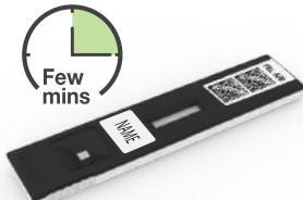
Leave the cartridge outside of the analyzer. Wait for the required time.
