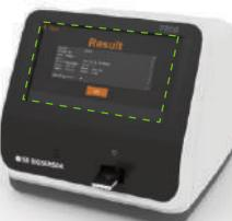
Insert the cartridge into the analyzer. It will take less than 1 min for the result.
