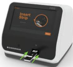
Insert the cartridge to initiate test processing.
